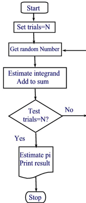
Figure 2. Flow Chart for estimating  $\pi$  using a finite integral.
