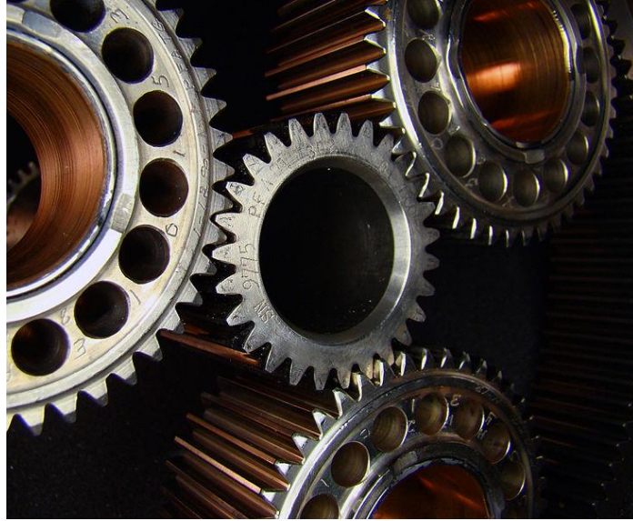
Figure 14. Pratt and Whitney PT6 turbine engine reduction gears (UH-1 Huey, DHC-6).
