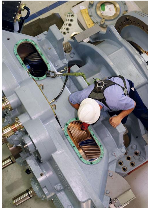
Figure 1. View inside a Liberty wind turbine transmission or gearbox.
