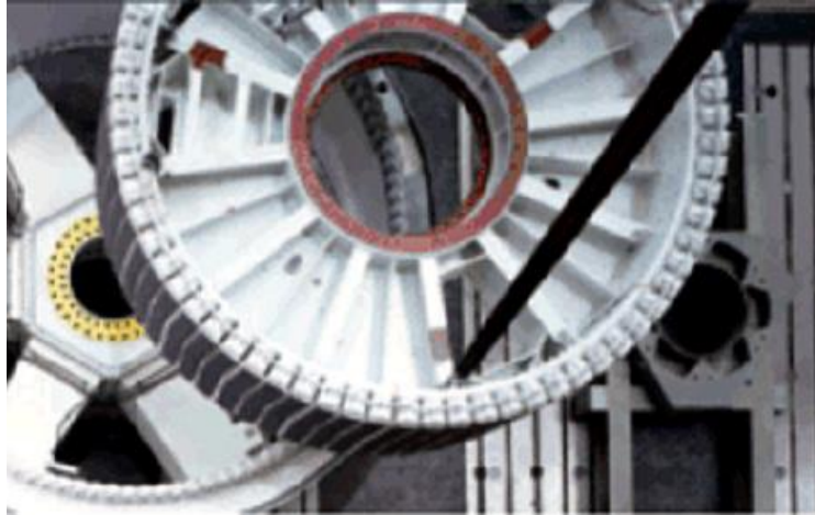
Figure 4. Stator and rotor of E-70 wind turbine. Source: Enercon.
