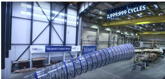
Figure 4. Fatigue loading testing for large wind rotor for offshore power generation.
