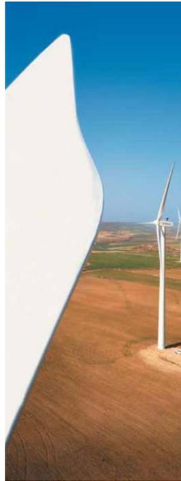
Figure 8. Tapered rotor tip to reduce the noise effect. Source: Gamesa.
