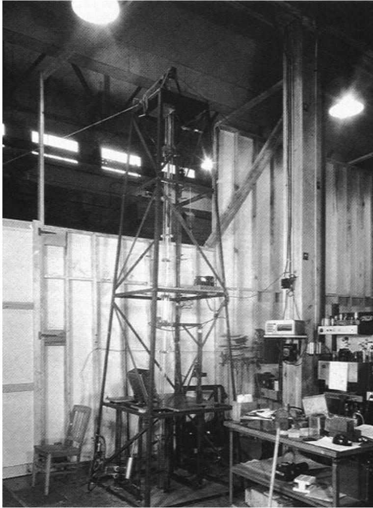
Figure 2. Guillotine setup to test the criticality of subcritical and critical configurations.
