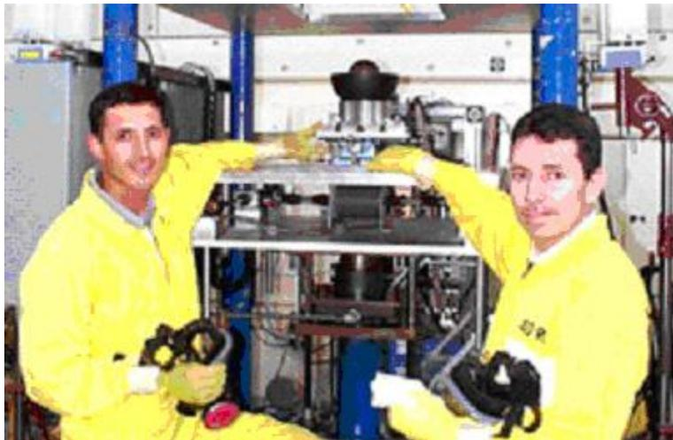
Figure 6. Modern Assembly machine at Los Alamos National Laboratory conducting criticality studies on a Neptunium<sup>237</sup> reflected with shells of highly enriched U<sup>235</sup>.
