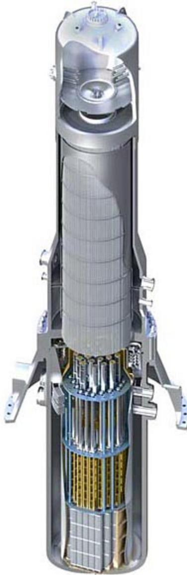
Figure 3. Integral configuration of core and steam generator within the reactor vessel of the modular reactor. Source Babcock & Wilcox.
