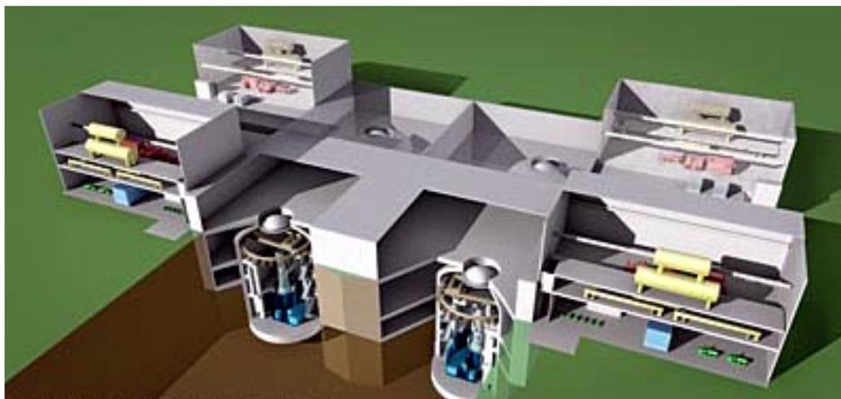
Figure 2. Compact Underground Reactor in a 4 units 500 MWe configuration of 125 MWe each.
