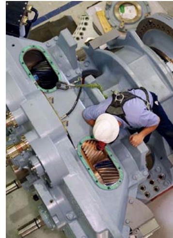
Figure 1. View inside a Liberty wind turbine gearbox. Source: Liberty.
